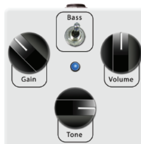
How to Drive a Plexi Gain at 10 o'clock, Tone at 3 o'clock, Bass Boost Toggle ON
