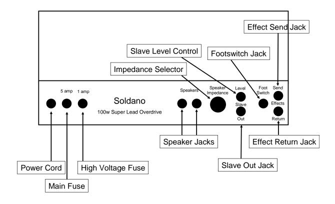
4. Plug in the Power Cord. Turn the Power Switch 'On.' Allow thirty seconds for the tubes to warm up. Connect a cord (either a speaker
