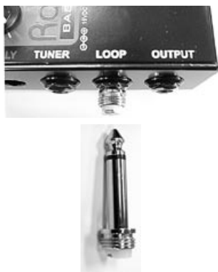
1/4" plug with solder leads trimmed off and shell removed.
