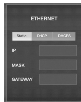
Mixer name and Ethernet setup screen
