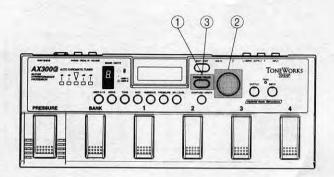
① When you finish editing a program (including settings for Pressure pedal, NR reduction gain, and total level), press and hold the Compare/Write key for 2 seconds or more. The upper line of the LCD display will show **PROGRAM WRITE**. The source program number will be shown at the left side of the lower line, and the destination program number will be shown at the right side.
