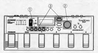
① In Play mode or Edit mode, press an IPE key. The upper line of the LCD display will show the selected IPE name, and the lower line will show the effect name. (The effects selected by the [DRIVE] and [TONE] IPE keys are for block 1, and the effects selected by the [MOD] and [AMBIENCE] IPE keys are for block 2.)
