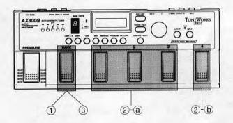
① In Play mode, select a program. Then press and hold the Bank switch for longer than 1 second, waiting until the blinking Bank/Note display changes to being steadily lit. The LCD display will change to the Individual On/Off pege, and will indicate INDIVIDUAL MODE.
