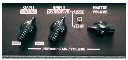
GAIN I increases the gain amount as you rotate the knob clockwise. As the gain increases, the tonal balance is shifted from a treble and upper mid emphasis, which produces an up front sparkling tone, to a lower mid and bass emphasis, which produces a thick meaty tone.
