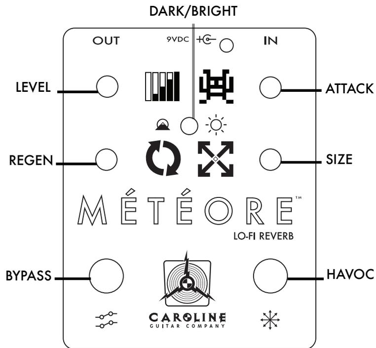
ATTACK sets the amount of gain in the preamp, allowing you to boost or overdrive the reverb. SIZE establishes the initial reverberation. REGENERATION extends the decay and adds overtones; set both this and SIZE high and the pedal can run away and self oscillate. LEVEL is the overall volume of the effect relative to your original signal. The DARK/BRIGHT toggle sets the overall voice.
