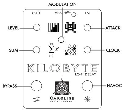
ATTACK adjusts the gain in the repeater preamp, allowing you to boost or overdrive the echoes. CLOCK sets the amount of delay time. SUM is the number of repeats; set this high and this pedal can run away and self oscillate. LEVEL is the overall volume of the repeats relative to your original signal. MODULATION controls a gentle amount of pitch shifting in the repeats. It was designed for us by our friend Jack DeVille at Mr. Black Pedals.
